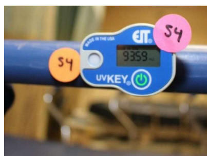
The EIT 2.0 UVKey can be used to easily confirm the numerical dose value of UVC in an operating room (left) and in high touch patient areas such as a bed rail (above)
